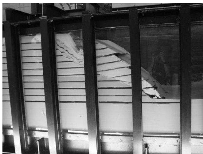
Fig. 6. Slope body and shear plane after failure. The actual measurements of this specific demonstration experiment were not used in the evaluation because the colored sand slightly changed its behavior.
